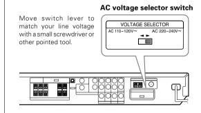
Note: Our warranty does not cover damage caused by excessive line voltage due to improper setting of the AC voltage selector switch.
