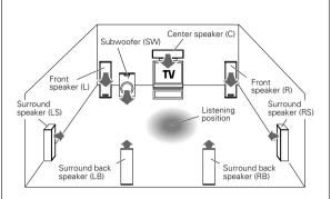
**Front speakers**: Place the left and right speakers at each side of your TV. Angle the speakers towards the listening area to enhance the stereo effect.
