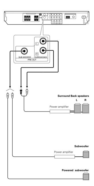
Connecting a speaker cord directly to a PRE OUT jack will not produce any sound from the speaker.
