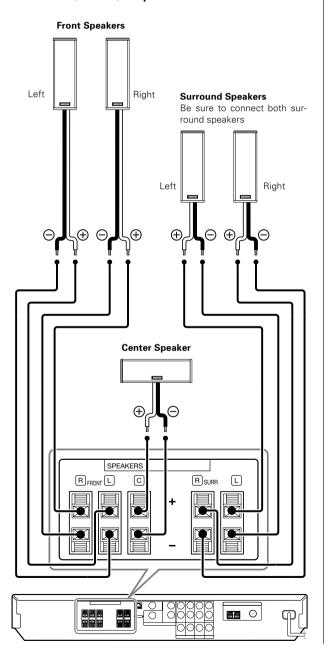
Whether each speaker is connected properly can be confirmed by outputting the test tone and checking if each speaker channel outputs audio. For details, see "Speaker settings" (Step Adjust the speaker volume level).
